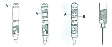
Single Check Single Valve Bailer. Includes a Dome Design polyethylene top (A) to avoid hang ups during bailer retrieval and retain the ball for top emptying. Dome Design bottom avoids hang ups when lowering the bailer. Also includes slide-in, angle-cut nozzle (B) for easy sample removal. Available in .75", 1.5" and 3" ID.
